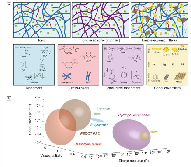
Figure 1. Hydrogels: (a) Schematic illustration of the main building blocks forming hydrogels and conductive hydrogels. (b) Quantification of the elastic modulus, electrical conductivity, and viscoelasticity (tan(δ)) of various tissues and conductive composites. CNT, carbon nanotube. Adapted from Reference 15.
