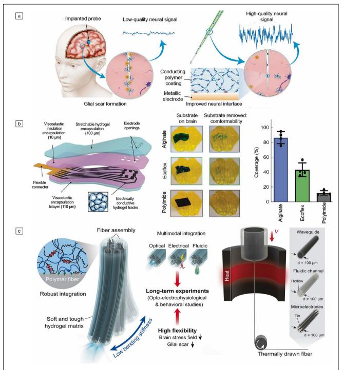
**Figure 3.** Examples of multifunctional hydrogels leveraging biological, mechanical, and electrical properties for implantable neuroelectronic interfaces. (a) Conductive hydrogel for electrode coating.<sup>89</sup> (b) Soft electrode array entirely prepared with viscoelastic materials.<sup>88</sup> (c) Adaptive, multifunctional hydrogel-based probe for the brain.<sup>11</sup>
